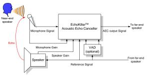
Fig. 1: EchoKiller's block diagram
